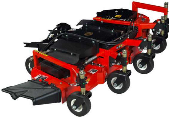
The Steiner Flex Deck is an adaptable mowing attachment fabricated with four hinged, floating decks and four blades to provide even mowing on the undulating, hilly terrain found around tee boxes, water hazards, bunkers and rough. This flexible mowing attachment features an 80-inch overall cutting width, a 1.5-inch to five-inch height of cut range and seven caster wheels for added support.
